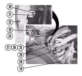
h. Remove coil spring (30) coil spring bushing (31) from spring perch (17) and lower a-arm (10).
