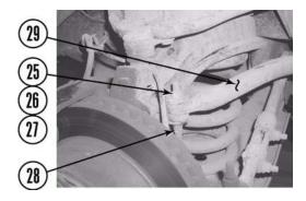
f. Remove lower shock bushing (16) and washer (15) from shock (13)
