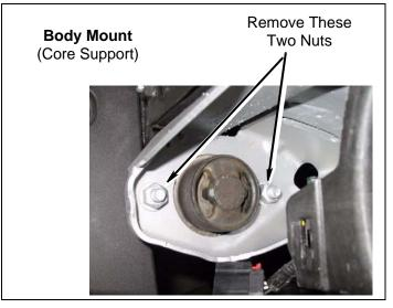
d. Passenger Side: Remove bolt and lower bushing from each cab mount on passenger side. 2 **Door** - 4 body mount bolts and **4 Door** - 5 body mount bolts.
