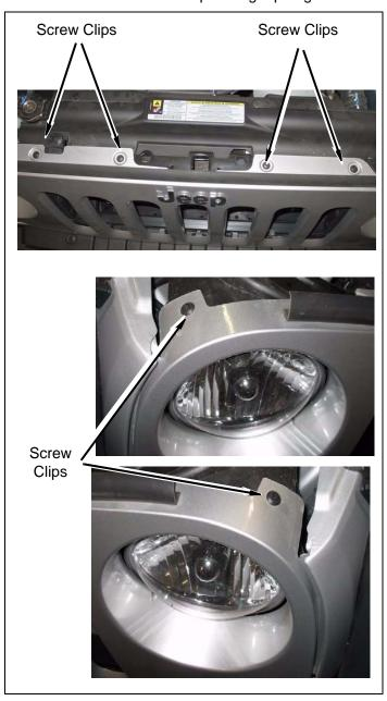
**c.** Remove grille from vehicle by popping four clips along bottom of grille.
