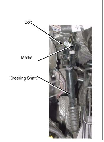
**c.** Remove bolt and slide u-joint off of steering shaft.
