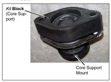
f. Install four *kit* washers (10 mm), two *kit* bolts (10 mm x 50 mm), two nuts (10 mm) and core support mount on vehicle.
