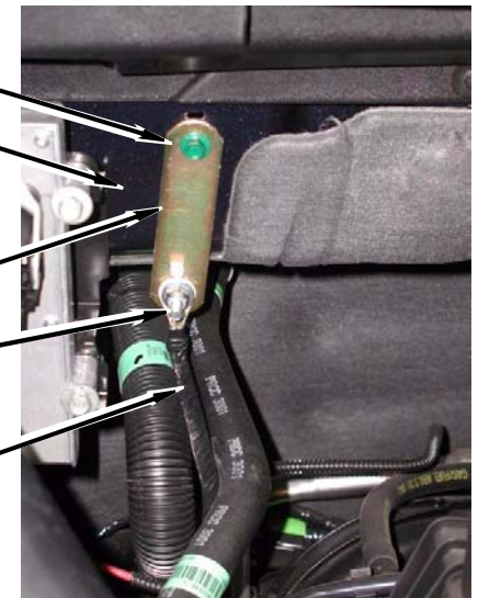
Bolt Firewall Kit Bracket (flat, 4", with 1/4" stud) Kit Nut (1/4" Nylock), Washer (1/4") Ground Strap
