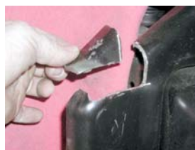
Mark and cut the frame horns (passenger side is shown)
