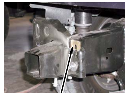
Temporarily install the kit bracket to ensure it lays flat against the frame horn (driver side is shown)
