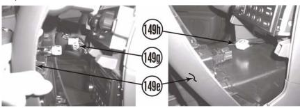
d. Install dash console cover (149e) on dash (149f) with four screws (149c) and four clips (149d).
