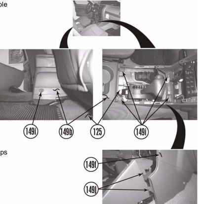
f. Lift storage console (149b) and locking clips (149j) from dash (149f).
