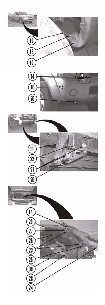
c. Remove bolt with captive washer (31) from air cleaner housing top (30).
