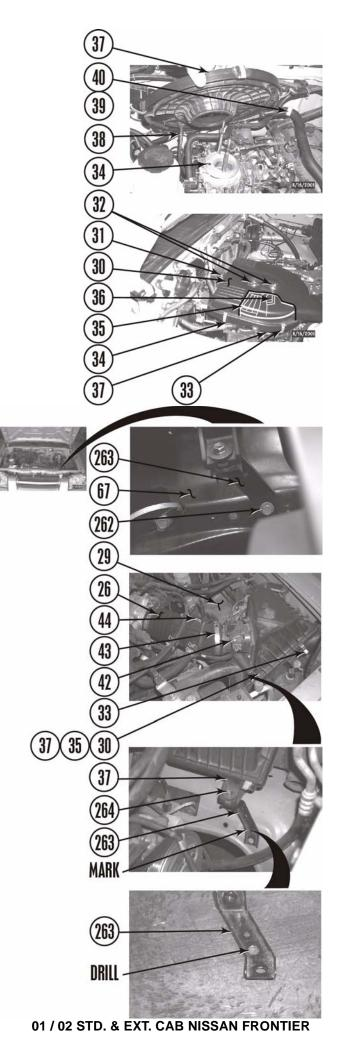
f. Install bracket (263) on lower air cleaner housing (37) and driver side wheel well (67) with two bolts with captive washers (262 and 264) as shown.
