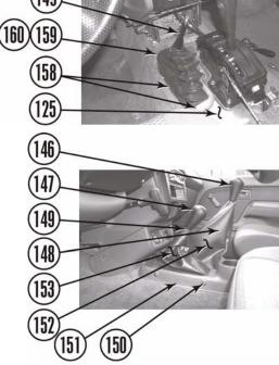
b. Install storage console (149b) on cab (125) with six screws (149i).
