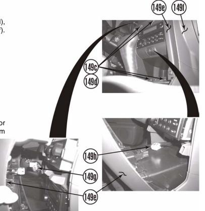
d. Disconnect emergency flasher wiring connector (149g) and lighter wiring connector (149h) from dash console cover (149e).
