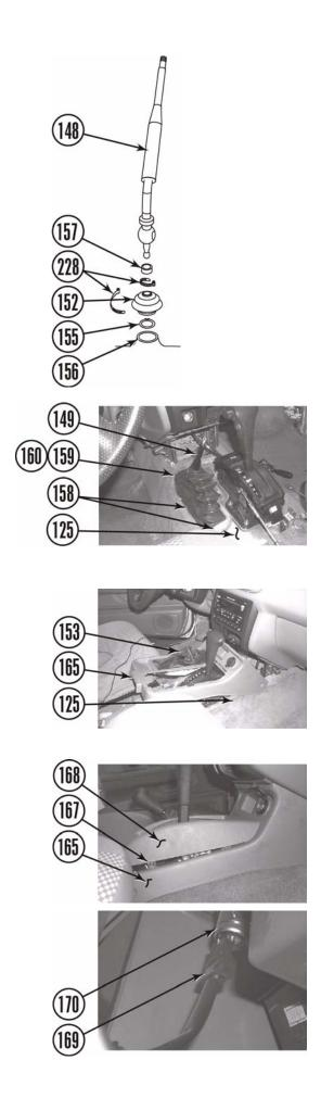
e. Install rear console (166) and 4wd with automatic transmission console (165) on cab (125) with eight screws (150).
