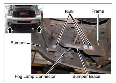
c. Remove two bolts from each fender side and remove bumper face from core support and fenders.
