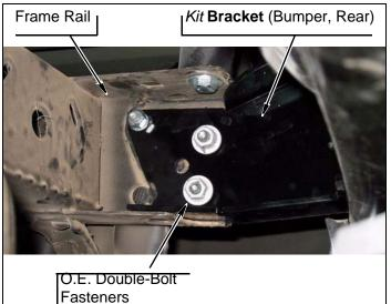
**h.** Mark eight holes through two *kit* **brackets** (bumper, rear) onto bumper support.
