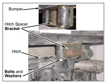
r. Adjust bumper to bed clearance using measurements taken earlier and tighten hitch bolts first then remaining bolts and nuts to 55 lb-ft.
