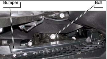
f. Install two *kit* **brackets** (bumper, front, support) onto bumper with two *kit* **large washers** between bumper and kit bracket. DO NOT TIGHTEN
