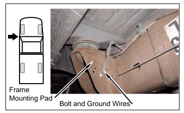
Pull some slack in parking brake cable. Clamp two cables at cable housing where indicated by arrows.
