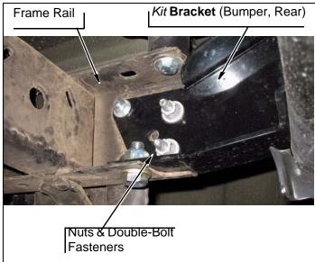
q. Install kit bracket, hitch spacer, on rear bumper and hitch with two kit bolts (14mm x 110mm) and two kit washers (14mm). Do not tighten.
