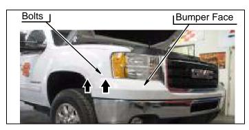
b. Position grill on core support and install six clips and four bolts in core support and front fenders.
