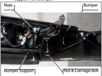
**d.** Cut two brackets and remove from bumper support as shown.
