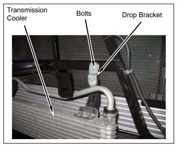
b. Install two *kit* **Spacers** in between lower transmission cooler bracket and core support using *kit* (3/8 x 2 1/2") hardware.
