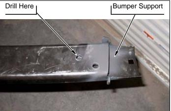
I. Install bumper support onto two *kit* brackets (bumper, rear) with four *kit* bolts (1/2"-13 x 3"), eight *kit* washers (1/2" SAE) and four *kit* nuts (1/2"-13 Stover). DO NOT TIGHTEN.
