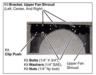
i. Using kit **bracket**, **upper fan shroud** (center) as template, drill two 1/4" holes in fan shroud lip. Install kit **bracket**, **upper fan shroud** (center) on upper fan shroud lip with two kit **clips push**.
