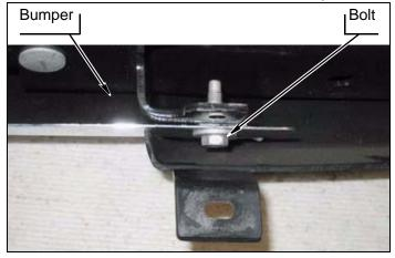
**c.** Remove six nuts, two carriage bolts and bumper support from bumper.
