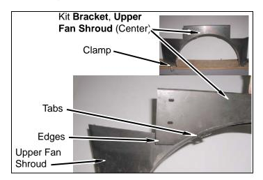
d. Assemble three kit **brackets**, **upper fan shroud** (left, center, and right) with two kit **bolts** (1/4" x 3/4"), four kit **washers** (1/4" SAE), and two kit **nuts** (1/4" nylock) as shown. Snug, bolts but do not tighten.
