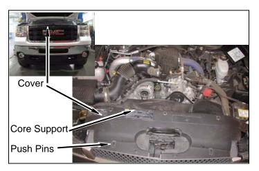
b. Remove four bolts, six clips, and grille from core support. Some GMC models may have extra clips.
