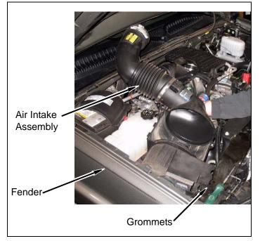
b. Tighten clamp on air intake assembly. Install wire harness clip on sensor.
