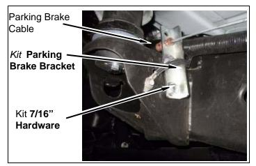
c. Install two ground wires on frame mounting pad with bolt. Connect front and rear brake cables. Remove clamps from rear cable. Note: *Kit* washer may be used between *kit* bracket and body mount to keep bracket aligned.
