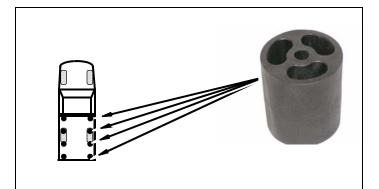
c. Install kit lift **blocks** on frame and bed with four kit **bolts** (12mm-1.75 x 100mm) and four kit **washers** (7/16" USS). Do not tighten.
