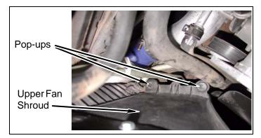
d. Remove computer wiring harness from harness push clip and lower fan shroud.
