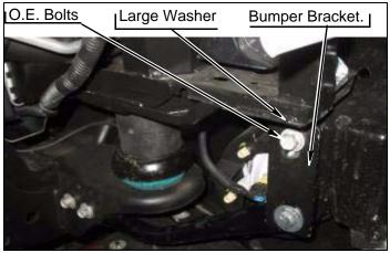
**g.** Install two bumper supports onto kit brackets with two *kit* **bolts** (7/16"-14 x 1-1/2"), four *kit* **washers** (7/16" SAE), two *kit* **nuts** (7/16"-14 Stover) with four O.E. bolts to body mount. DO NOT TIGHTEN.
