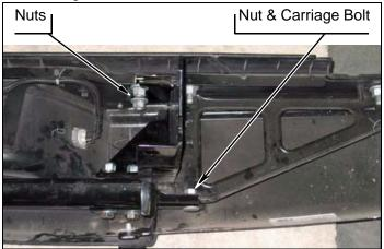
**n.** Install bottom of bumper onto bumper support with two bolts.
