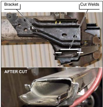
e. Position two *kit* **brackets** (bumper, rear) onto bumper support against stop.
