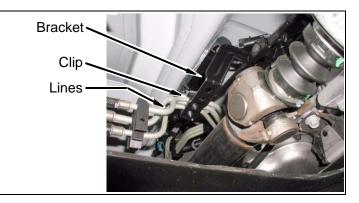
b. Remove two nuts and bracket from transfer case. <u>Bracket is not reused.</u> Install two nuts and tighten.
