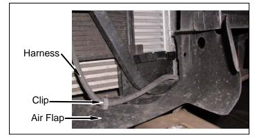
d. Remove two clips, three push pins, and air flap from core support.
