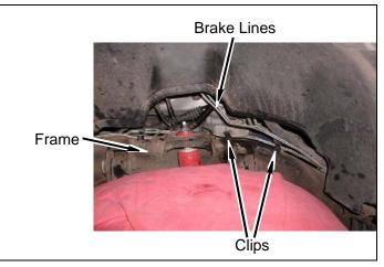
c. If possible, install harness in clip on frame driver side.
