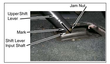
c. Loosen jam nut and remove upper shift lever from shift lever input shaft.
