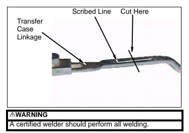
c. Position kit **pin** 4x4 extension between two pieces of transfer case linkage. Ensure transfer case linkage scribed lines align and weld kit **pin** extension in place.
