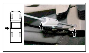
c. Separate front parking brake cable from rear parking brake cable at cable connector.
