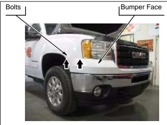
**d.** Remove four nuts, two double-bolt fasteners and two frame brackets from two frame horns.
