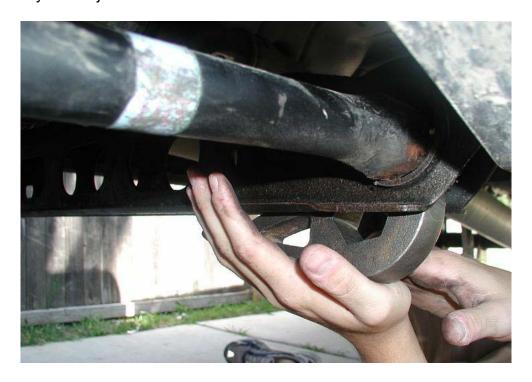
Try to center the key in the crossmember – the more centered it is the easier it will be to slide the torsion bar back into the key. Slide the torsion bar into the crossmember and into the torsion lift key. Make sure the torsion key is centered in the crossmember once the torsion bar has been inserted. Place the puller back onto the crossmember and insert the threaded end of the puller back into the dimple of the new torsion lift key.
