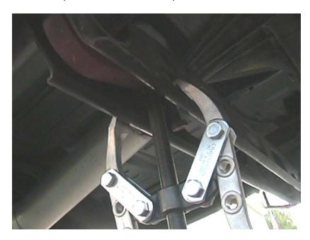
Using an 15mm or 18mm socket you can remove the stock adjustment bolt by turning it counter-clockwise until it is easily removed. !!! CAUTION !!! AVOID USING YOUR HANDS TO REMOVE ITEMS – IF THE PULLER SLIPS YOU COULD SERIOUSLY INJURE YOURSELF – USE PLIERS AND KEEP A SAFE DISTANCE FROM THE PULLER AND CROSSMEMBER WHEN REMOVING THIS BOLT!!!
