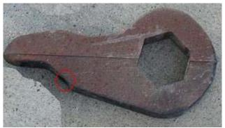
(The red circle indicates a dimple on the key. This dimple is where you locate the tip of the unloading tool.)
