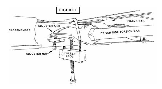
This cutaway illustration shows an alternate method to properly remove and install a torsion key.
