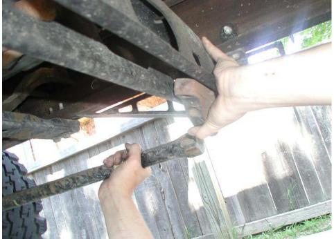
4) INSTALLING YOUR NEW TORSION LIFT KEYS... Installation of your new keys is the reverse of removal. If the torsion bar slid to far forward during removal of the key now is the time to guarantee it
