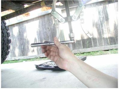
Continue to tighten the puller (pushing against the torsion lift key) until it is possible to re-install the adjustment bolt holder back into the crossmember. \*\*\* CAUTION \*\*\* – DO NOT USE YOUR HANDS
