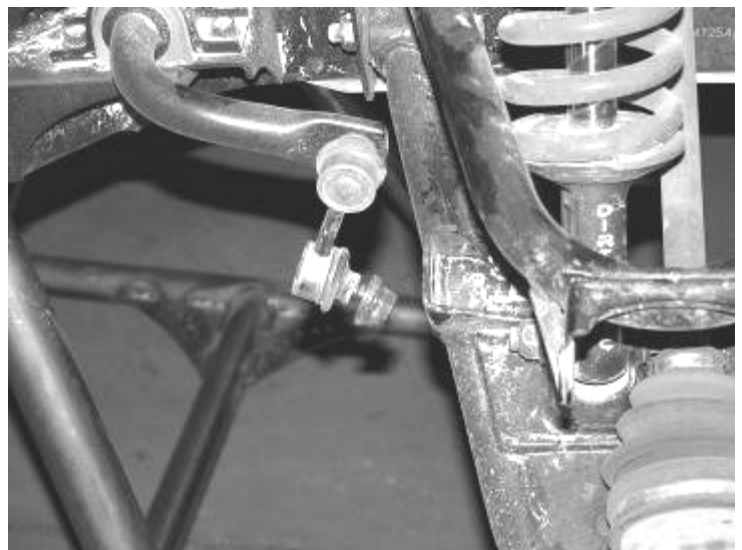
44. Remove the upper control arm and save the hardware. SEE PHOTO BELOW
