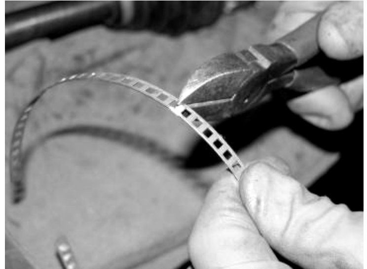
17. Using a CV boot band clamp tool, clamp only the inner boot clamps. Locate one of the supplied CV boot grease bags ( 4 bags are provided with this kit, one for each axle, half a bag for each CV ). Carefully pull back the boot from the inner CV and insert HALF of the bag into one inner CV boot. Re-install the boot onto the CV and use the clamp tool and tighten the clamp. Repeat this step for the outer CV. SEE PHOTO BELOW
