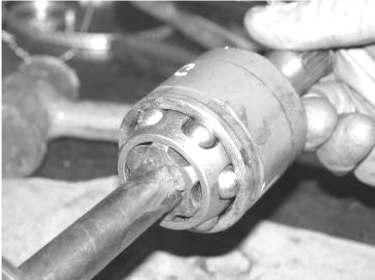
15. Locate the Inner CV housing and factory large snap ring (one wire style). Install the housing onto the axle over the CV cage and install the large snap ring. Slide the CV boot over the CV and Housing. SEE PHOTOS BELOW AND ON NEXT PAGE
