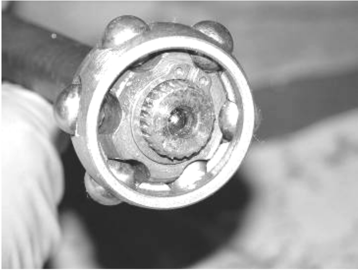
15. Locate the Inner CV housing and factory large snap ring (one wire style). Install the housing onto the axle over the CV cage and install the large snap ring. Slide the CV boot over the CV and Housing. SEE PHOTOS BELOW AND ON NEXT PAGE
