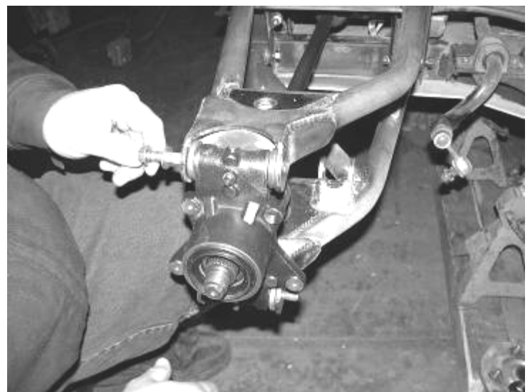
54. Locate and install the factory hub assembly onto the knuckle and axle shaft. Install the factory axle shaft nut and torque to 190 lbs. (use supplied thread-locking compound) Use a center punch and re-crimp the hub nut in the key way of the axle SEE PHOTOS IN NEXT COLUMN.
