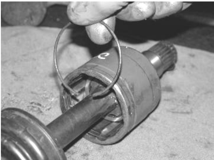
16. Locate two large and two small CV boot clamps from the FT95060 clamp kit. Position the large clamp around the boot
