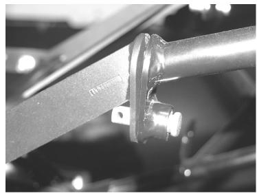
6. Locate FT95093BK support bracket clamp. Use the 5/16 bolts, nylock nuts and washers to fasten the support bracket. Torque to 14 ft. lbs. SEE PHOTO ON NEXT PAGE.
