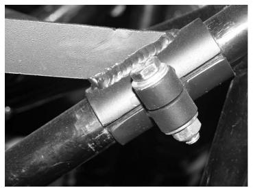
7. Tighten the support bracket driver and pass. Torque to 14 ft. lbs. SEE PHOTO BELOW.
