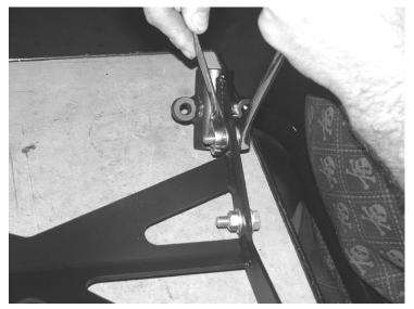
5. Line up the two holes in the bumper with the two holes in the support bracket leaving an 1/8 space between the two. Place the 3/8 clevis pins through the two to keep them inline. SEE PHOTO BELOW.
