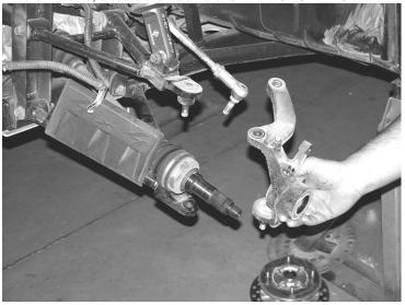
5. Place the knuckle into a vise with aluminum or soft jaws and use care not do damage. Use a drill with a ¾" drill bit and drill out the knuckle at the tie rod location. SEE PHOTOS BELOW
