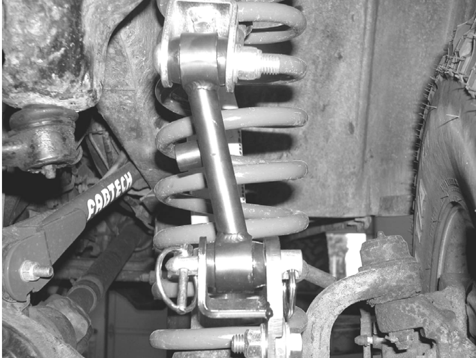
Note The Offset Of The Sway Bar End link (Driver Side Shown)
