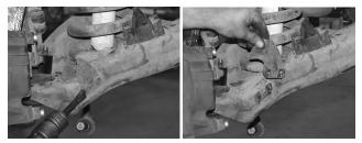
16. Using an air chisel, remove the 2 rivets securing the steering stop to the lower control arm.
