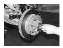
11. Place a light coat of grease onto the axle and slide the rotor on. Reinstall the original nut. Tighten the castle nut just enough to remove any free play from the rotor and still allow it to rotate freely. Insert the cotter pin retainer and one of the new cotter pins. Tap the dust cap back in place using a rubber mallet.
