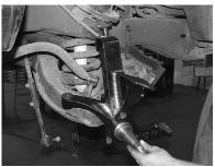
8. Take the driver's side spindle, marked FT2588-7D, and install it onto the upper and lower ball joints. Reinstall the original castle nuts and torque to factory specs. Install a supplied cotter pin in each castle nut, **DO NOT REUSE THE ORIGINAL COTTER PINS.**
