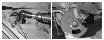
5. Unbolt the abs line clamp from the top of the frame and disconnect the wire connector. Open the wire clamp holding the ABS line onto the bottom of the upper control arm. Remove the 3 bolts securing the brake dust shield and ABS sensor (on late model trucks) to the spindle. Slide the shield off the spindle.
