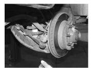
3. Remove the nut securing the tie rod end to the spindle. Separate the tie rod from the spindle using a tie rod end puller.
